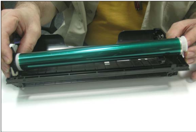
10. When the drum is extracted there will be a spring loaded clutch piece at one end and a drive gear on the other side coming loose.
