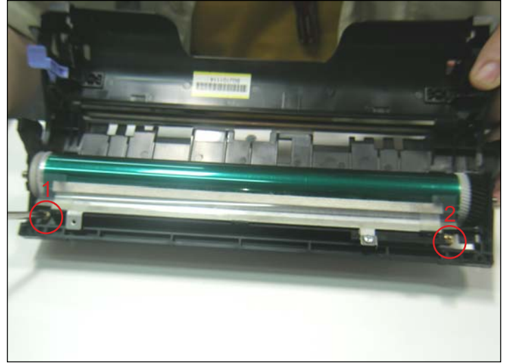
5. With a Phillips screwdriver remove the screws holding the drum cleaning assembly. You will notice that it is composed of a cleaning felt, a recovery blade and a couple of scraper-blades.
