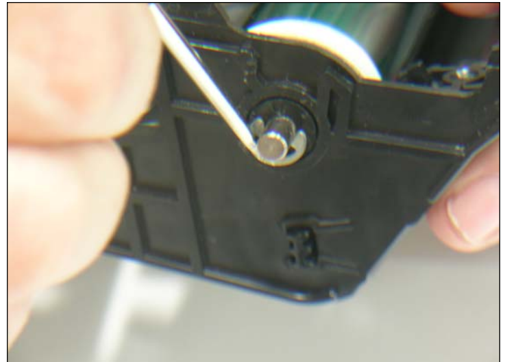
7. Remove the shaft of the drum by releasing the retaining washer from the left side of the cartridge.
