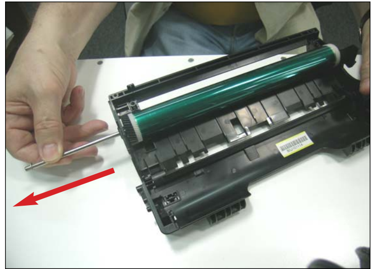
9. Slide the axle away from the cartridge as shown.
