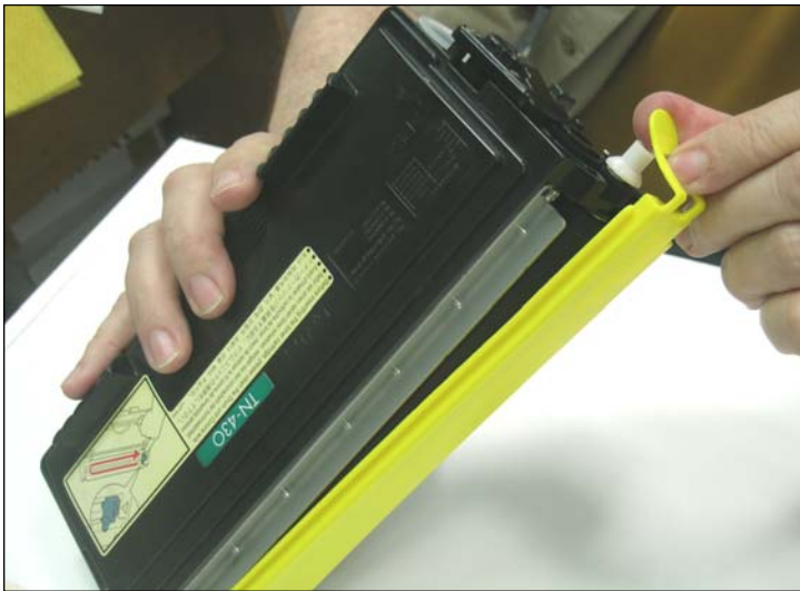
3. Insert the OEM or the compatible yellow seal cover for the developer roller to protect it during transit.
