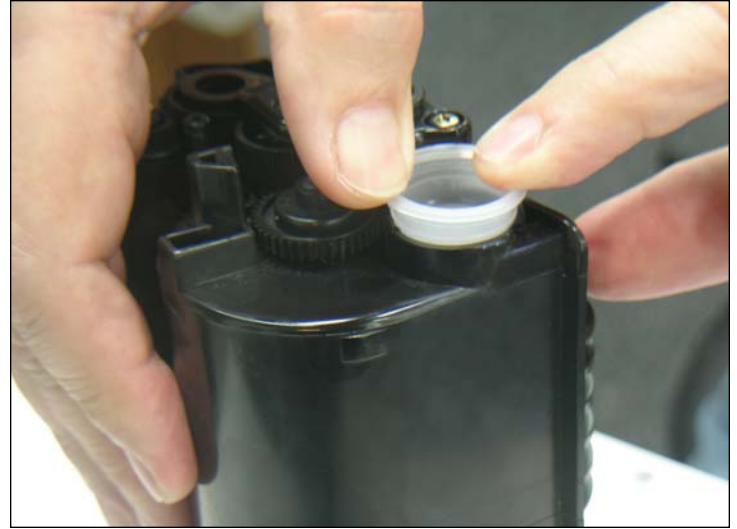
2. Recap the hopper securely.
