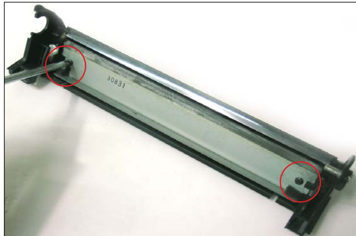
14. Remove the two screws that hold the wiper blade in place.
