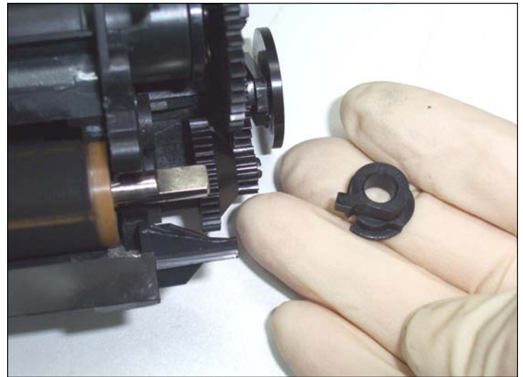
28. Developer roller shaft bushing removed.
