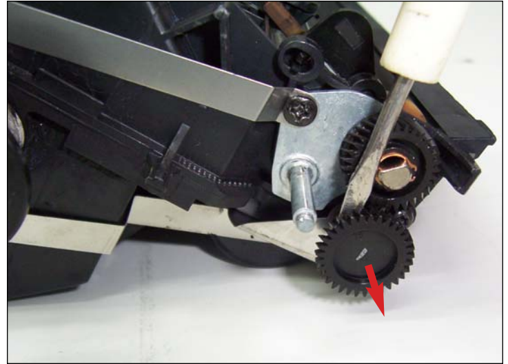
10. Push the supply roller gear (shown) out using a small flat-head screwdriver and applying a small amount of force.
