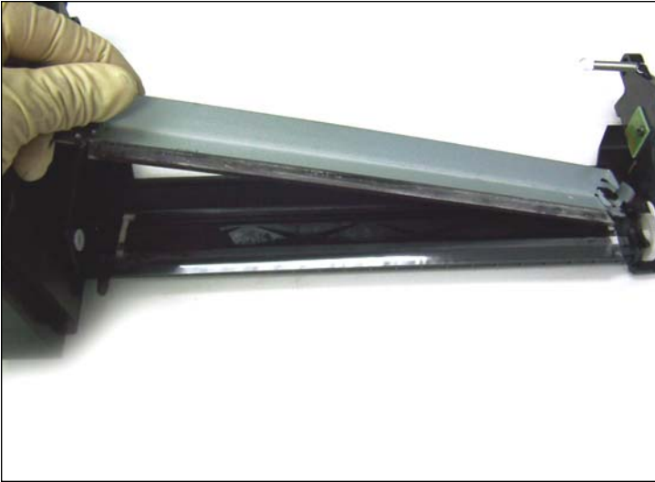
40. Lift the wiper blade and remove as shown.
