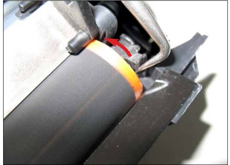
26. Next, unlock the developer roller shaft bushing by rotating it upward as shown using a hook tool.
