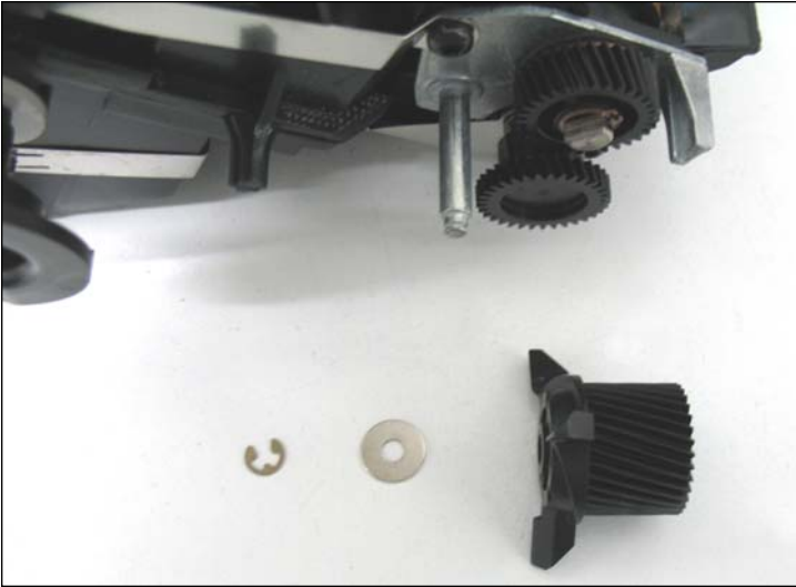
9. "C" clip, washer, and drive gear (shown) removed.
