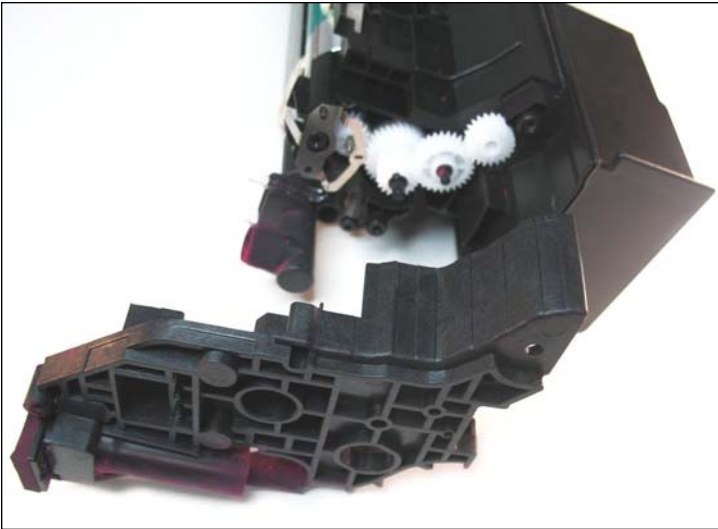
38. Once the chip has been installed, you can proceed with installing the inner section of the end cap.
