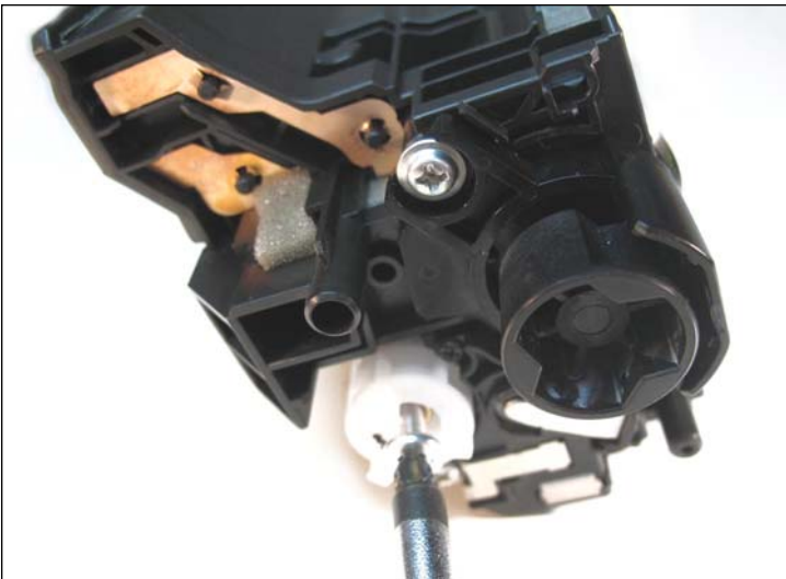
31. Install the developer roller drive gear and its appropriate screw.
