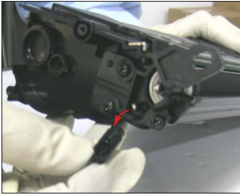
3. Remove the extension gear next to the developer roller on the gearless side of the toner cartridge.
