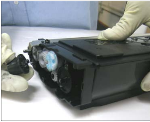
12. Remove the outer gear (black) as shown.
