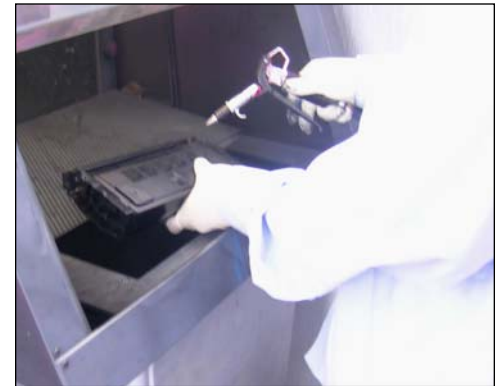
20. Clean cartridge thoroughly using compressed air or vacuum. Refill with 245 grams of toner M20 and reassemble cartridge by reversing the steps above. Before re-installing the gearside end cap a new Smartchip must be fitted.
