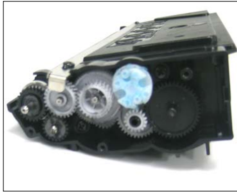
13. Remove the rest of the gears shown.
