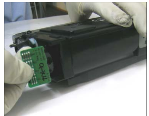
11. Remove chip as shown. It will be replaced later with a new Smartchip
