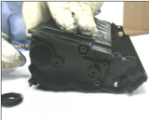
18. Using a pair of needle-nose pliers, pull out the toner fill cap (gearless side) to empty and clean the toner cartridge.
