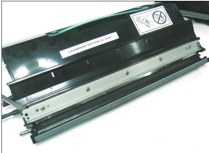
29. Using a flathead screwdriver, lift the doctor blade far enough to grasp with your hands.
