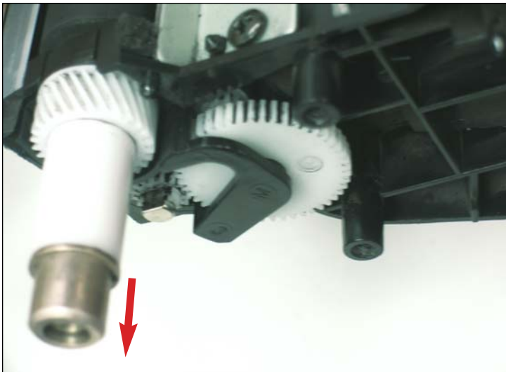
19. First, slide off the gear and brass bushing from the drive shaft as shown.
