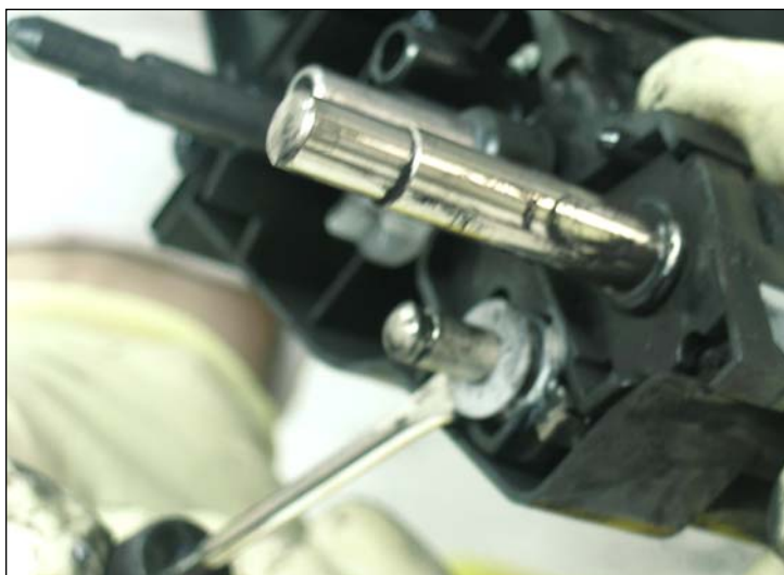
10. Using a small flat-head screwdriver, remove the Supply Roller Gear Washer shown.
