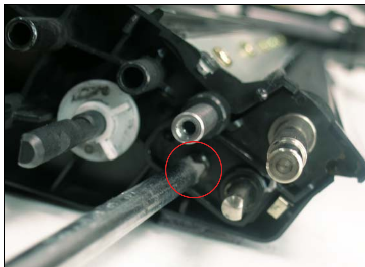
12. Remove the screw that holds the gear housing in place.
