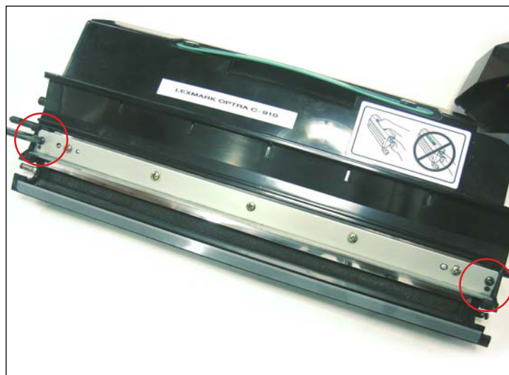
28. Remove the two screws on shown that hold the doctor blade in place.
