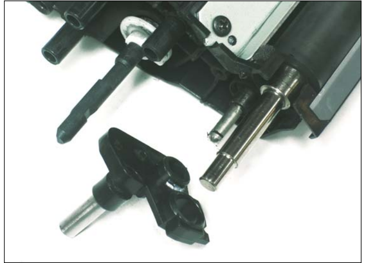
14. Gear housing removed.
