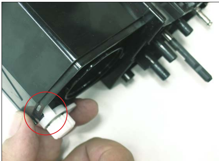
REMOVING THE WASTE TONER HOSE & SPRING GEAR 31. First, locate the interlocked gear next to the toner fill plug on the gear-side of the toner cartridge.
