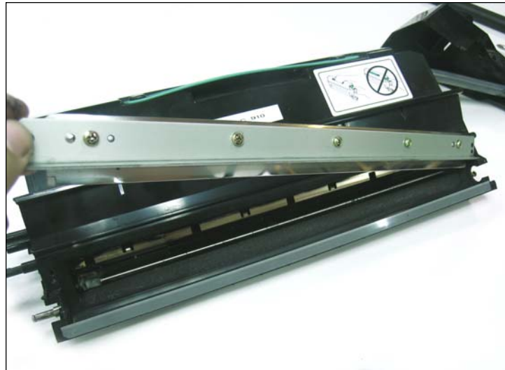
30. Lift the doctor blade out from one side, then to the next.
