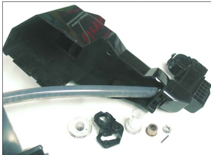
26. Make sure all end cap components are accounted for before continuing.
