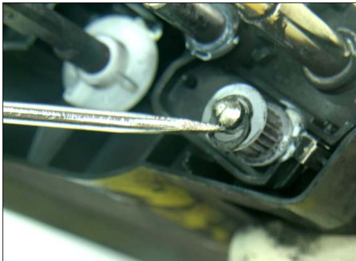
9. First, remove the “C” Clip that holds the Supply Roller Gear in its place.
