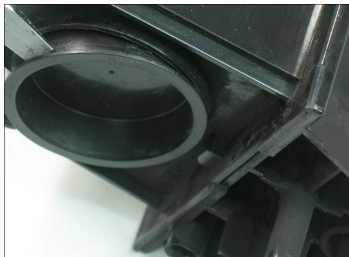
36. Using a flathead screwdriver, pry open the toner fill plug as shown.
