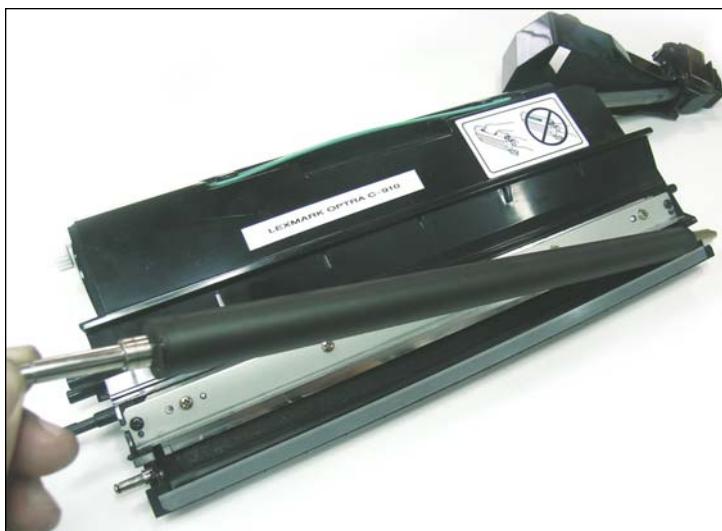
27. Lift the developer roller out from one side to the next.
