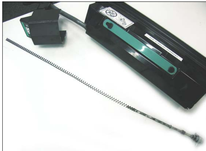
34. NOTE: The gear is attached to a long spring that runs through the toner hopper and hose attachment up to the gearless end cap. The spring should come out completely when pulled.
