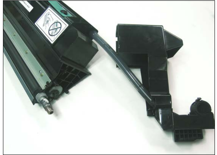
18. End cap separated from cartridge shown.
