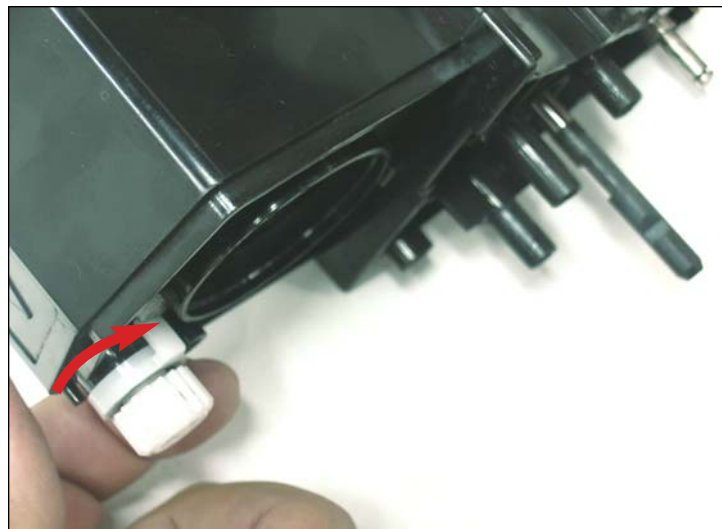
32. Turn the gear tab clockwise as shown to unlock it.
